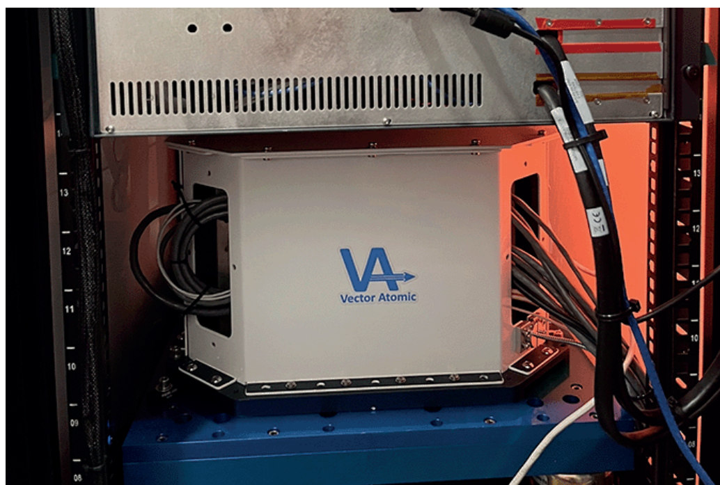
Figure 9: Vector Atomic Gravimeter
