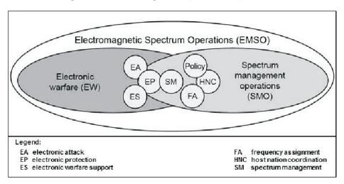
Figure 3. Electromagnetic Spectrum Operations
