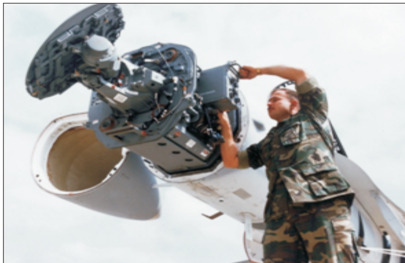
Mechanically-steered antenna on an F/A-18C/D undergoing maintenance (photo: Raytheon)
