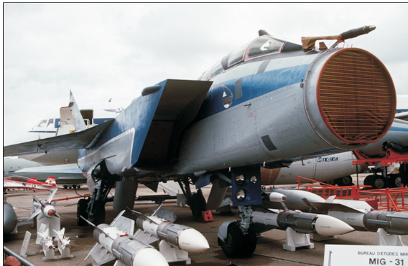
The Tikhomirov BRLS-8B 'Zaslon' was the first PESA to be installed in an aircraft—the MiG-31 interceptor (photo: USAF)
